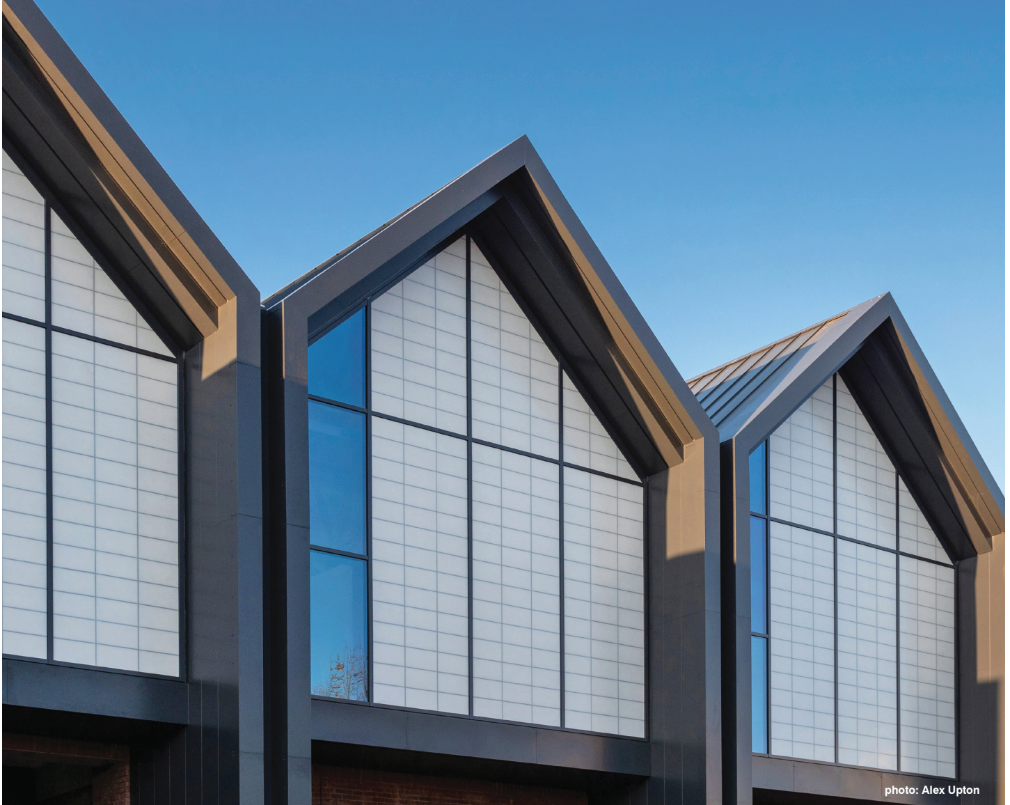
The Mall, Walthamstow | London, UK | ESA Architecture | KALWALL TIGUs mixed glazed in RAICO THERM+ Curtain Wall
